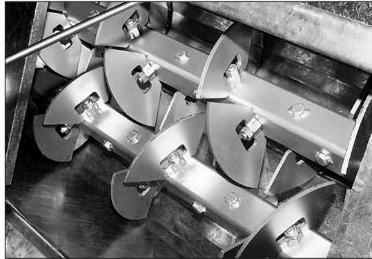
Fig. 4. Double shaft mixer with paddles [Borowski 2013d]
