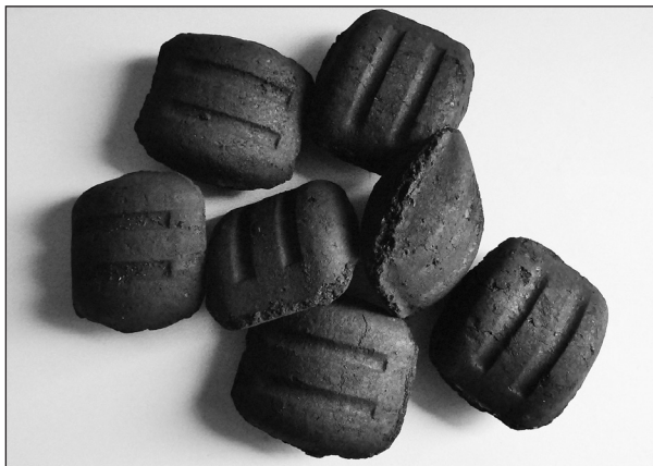
Fig. 16. View of the coal briquettes from the roller press (Phot. G. Borowski)
