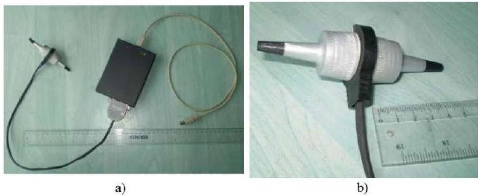
Fig. 6.37. External view: a) sensor device for flow measurement ; b) block of the primary converter
