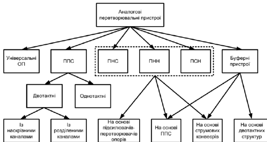
Fig. 2.2. Classification of the analog devices for the analog-to-digital systems
